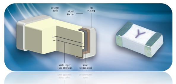
Fuse links and arc suppressing material are buried inside of fuse body. When fuse link opens, there is no fly arc or spark leak. Multiple fuse links design in parallel could improve the amperage rating and save board space. Fuse element diffused into ceramic body, so the integrity of fuse body is maintained and the airtight package is preserved.
