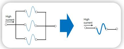
The CMF high power surface mount fuses build on AEM advanced manufacturing technology. The solid, robust structure assures reliable operation in environments where temperature cycling and high mechanical vibration are present. The devices singular fuse link/terminal construction eliminates problems that occur with traditional ceramic tube interconnection techniques
